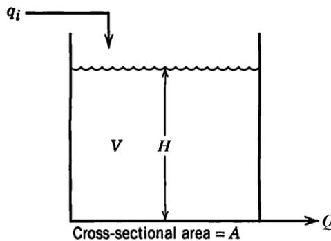
The height is measured in inches, and the outlet flow,  $Q$  is measured in liters per minute, and the inlet flow is  $q_i$ , a constant value. The variables  $Q'$  and  $H'$  are deviation variables.
