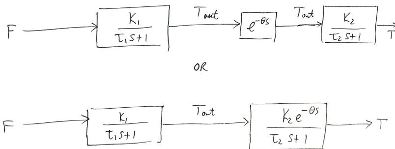
The time delay may appear either as a separate block, or merged with the second block.
