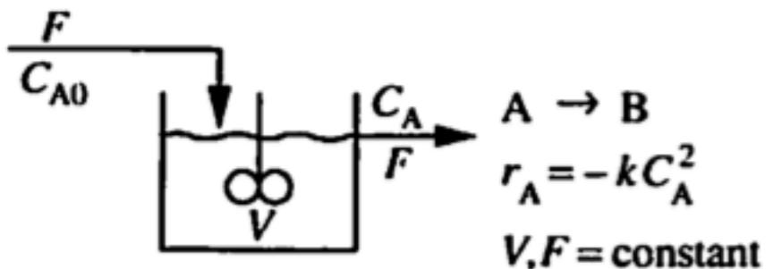
$$V \frac{dC_A}{dt} = F(C_{A0} - C_A) - V k C_A^2$$
