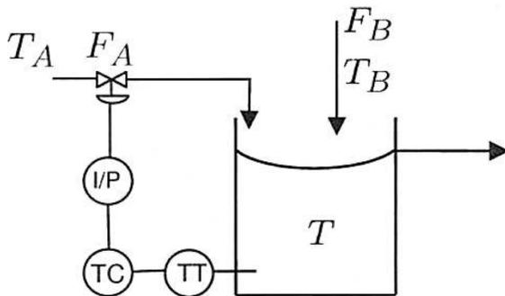
$$\text{An energy balance on the tank gives: } T'(s) = \frac{18}{2s+1} F_A'(s) + \frac{0.6}{2s+1} T_B'(s)$$
