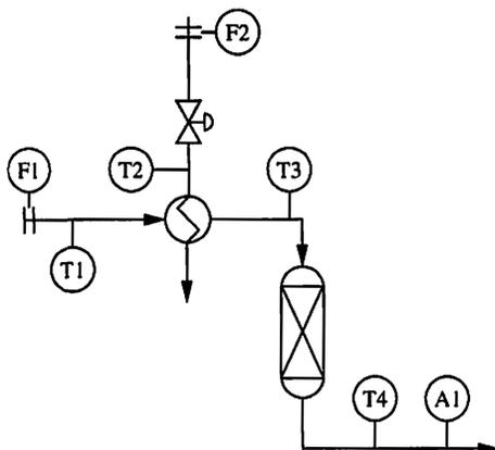
If the the (steam) valve position at F2 is opened 5% more (on the left axis), then the corresponding temperature output response at T4 is observed (right axis)
