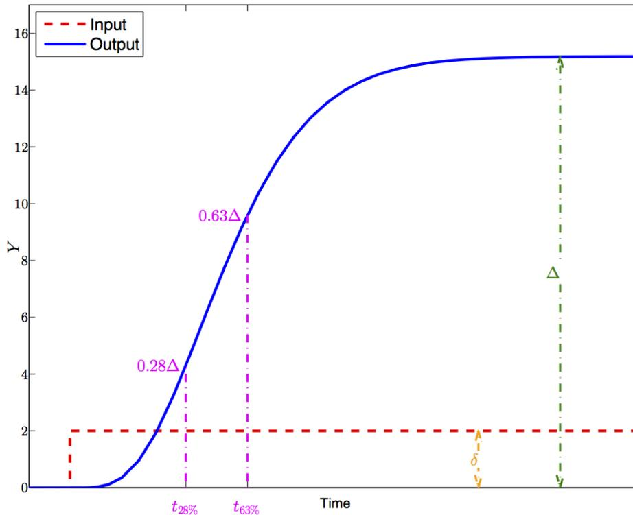
3. Find the points where the response is at 63.2% and 28.4% of the full response. These occur at  $t_{63} = 21.7$  seconds and  $t_{28} = 14.2$  seconds into the simulation from the point at which the step input was made. So then  $\tau = \frac{3}{2} [21.7 - 14.2] = 11.3$  and  $\theta = 21.7 - 11.3 = 10.45$  seconds. The gain,  $K_p = \frac{15.187}{2} = 7.59$ .
