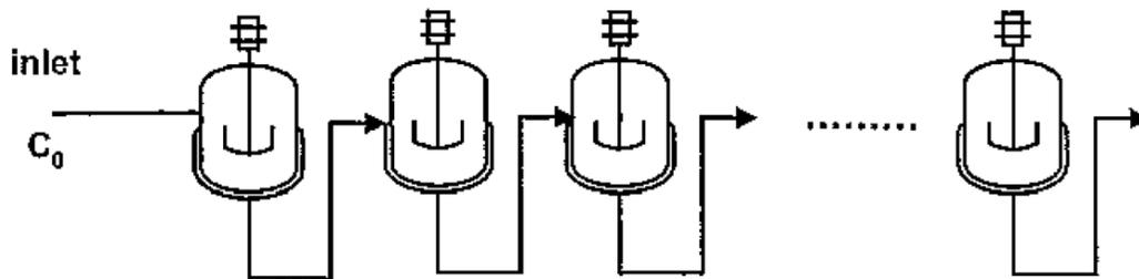
Consider tanks in series, each with a transfer function  $G_{p,i}(s) = \frac{X_{i+1}(s)}{X_i(s)} = \frac{K}{\tau s + 1} = \frac{1.5}{4s + 1}$ .
