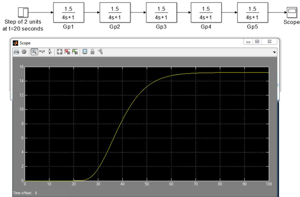
2. The gain of the system is found from the product of the transfer functions,  $\left(\frac{1.5}{4s+1}\right)^5$ , from which we can use the final value theorem with a unit step, and obtain  $K_p = 1.5^5 = 7.594$ . The gain is **not** the sum of 5 transfer functions,  $5 \times 1.5 = 7.5$  (though it is close).
