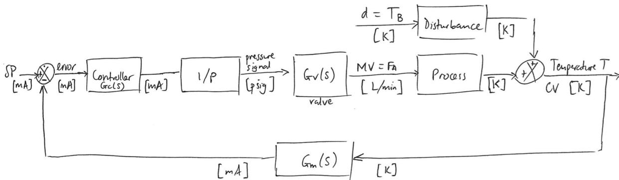
$$G_v(s) = \frac{0.5 \frac{[L/min]}{[psig]}}{0.1s+1} \quad \text{Disturbance } G_d(s) = \frac{0.6 \frac{[K]}{[K]}}{2s+1} \quad \text{Controller } G_c(s) = \text{unspecified}$$
