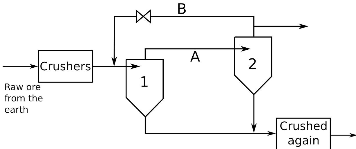
2. Assume the flow in stream B is zero (i.e. the valve in stream B is fully shut). What is the purpose of connecting cyclone 1 and 2 in series, using the connector stream A? [3]
