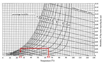
**Example:** Air at 65°C and 10% humidity has a dew point temperature of 25°C. This parcel of air contains 0.021 kg of water per kilogram of dry air.
