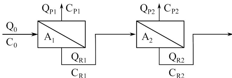
recognizing that it is the retentate from the first module that is fed into the second membrane.
