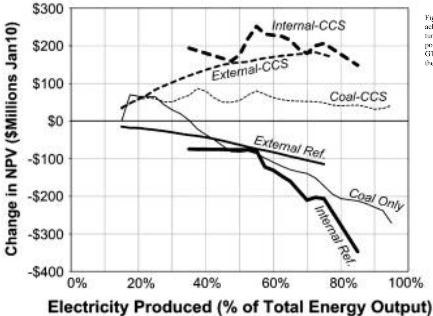
Fig.8 The change in the NPV achieved by switching from a gas turbine to SOFCs as the primary power generator (compared to GT-based cases as a function of the electricity production at t...
